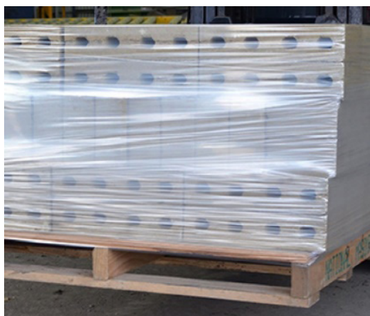
Figure 8. Third generation mLLDPE resins are being used in films requiring exceptional toughness.
